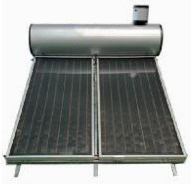
Hollandia HP Series thermo siphon system adopts the black anodized flat plate solar collector and solar storage tank with SUS304 as inner tank material. Both parts connect to each other directly. According to the thermo siphon principle, the water in tank is heated in continuous circulation.
